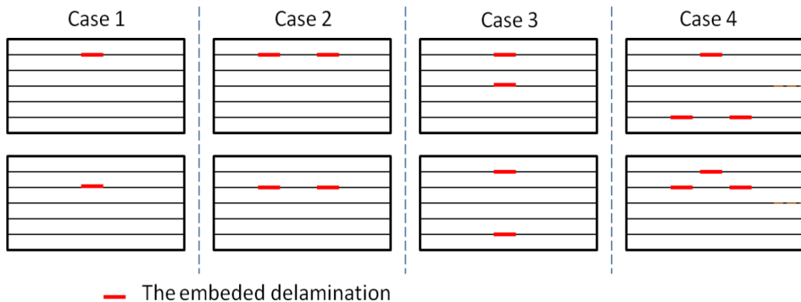
Figure 15. Different embedded delamination patterns
