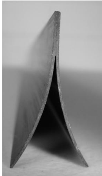
Figure 56. Cross section of AFRL composite boom
